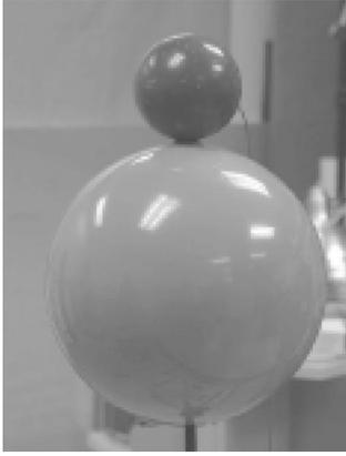
FIG. 2. The physical snowman model, which is composed of a 4.15-cm-radius bocce ball resting on top of a 10.9-cm-radius bowling ball. The probe tube microphone is inside the bocce ball, with the probe tip flush with the surface. The bowling ball is supported by a 0.5-cm-radius cylindrical rod.
